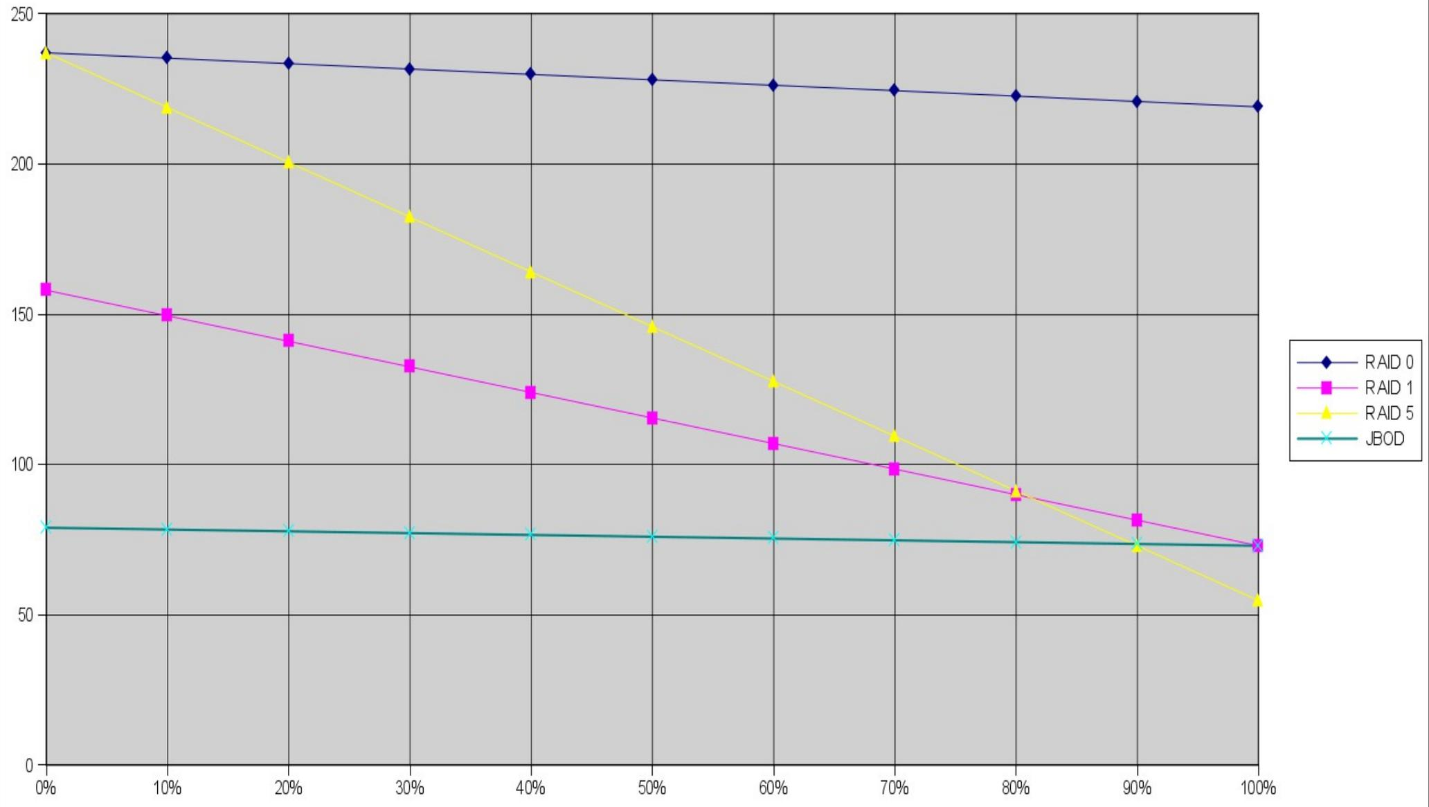
Here we compare a two disk RAID 1 array to a three disk RAID 5 array. RAID 5 manages to maintain a performance advantage.
