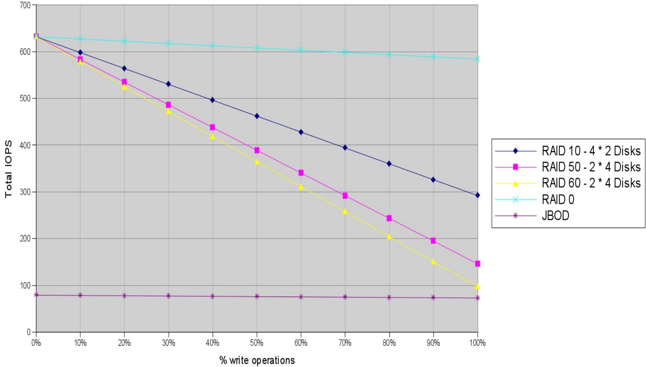
8 disk RAID 10 outperforms all other 8 disk RAID configurations
