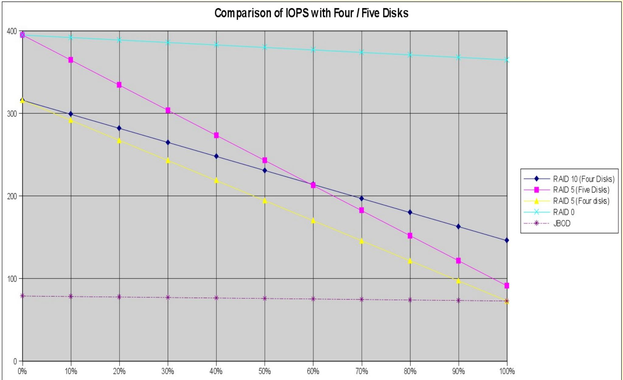
Here we compare a four disk RAID 10 array to a five disk RAID 5 array. RAID 5 works better, as long as the reads are light.
